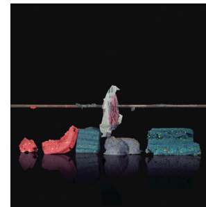
Integrity - Doesn't melt in hot conditions. Testing was conducted in an oven at 93°C for 8 hours.
